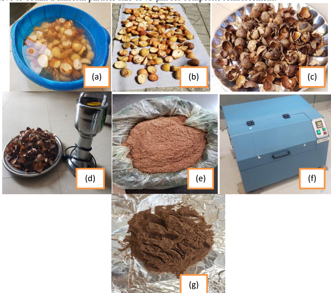
Figure 3.1: ASP preparation: (a): washed avocado seed, (b): drying the seed, (c): avocado cover peeled from the seed, (d): coffee grinder, (e): grinded ASP with coffee grinder, (f): Ball milling Machine, (g): milled ASP
