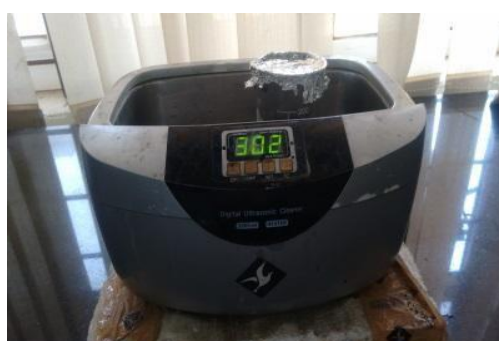
Fig. 2. Ultrasonication of MWCNTs using a bath sonicator.
